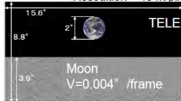
Figure 4. Schematic view of HDTV images for WIDE and TELE. 1920pixel x 1080pixel
