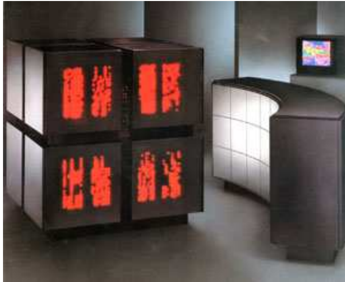
2048 floating point units in SIMD mode
